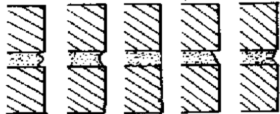
Grapevine, Concave, Flush, Raked and V mortar joints
